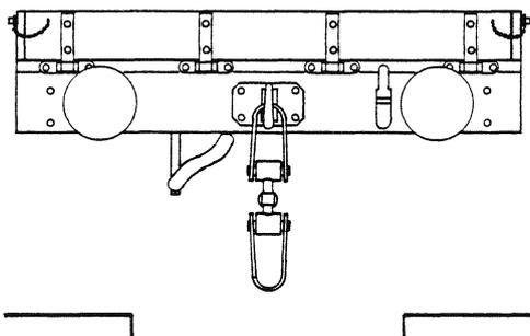
**LNER Livery.** Bodywork, Solebars & Buffer Beams - Red Oxide (RailMatch paints LNER freight red oxide No 625). Buffers, couplings, running gear and metalwork below solebars - black. Dirty wood floor planks. White lettering and white end of brake lever.
