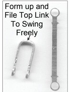
Pass the coupling hook through the slot and retain it with a length of spring wire. Polish the centre of this wire with emery cloth first so that you can solder it to the coupling hook shank once you are happy that the buffers spring freely.
