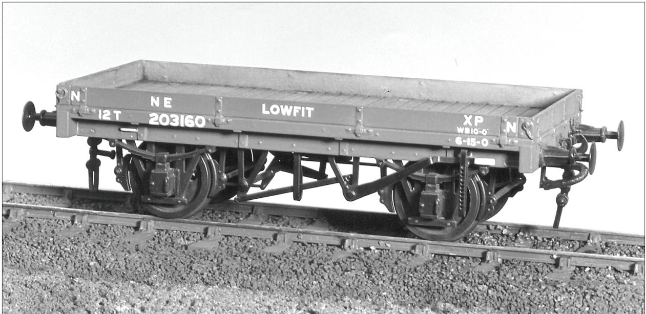
**PROTOTYPE.** In the mid thirties the LNER built nearly 1,400 single plank, vacuum brake fitted wagons with all four sides hinged at the bottom. They carried a large variety of loads but were particularly useful for small road vehicles such as farm tractors as with the end dropped they could be driven from an end loading dock onto the wagon.
